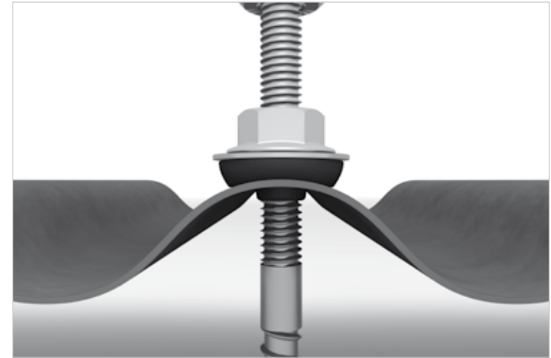
Detail illustration: Hanger bolt with FZD seal
